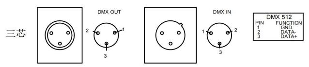
For the connection of control signals, 2-pin shielded cables with a diameter not less than 0.5 mm must be used between the fixture and the controller and between the fixtures. Please use the 3-pin signal output / incoming line of the lamp to connect. The connections between the 3-pin signal line ports are shown in the figure above. It must be noted that the 3 pin of the XLR plug / socket must not be in contact with the inner
