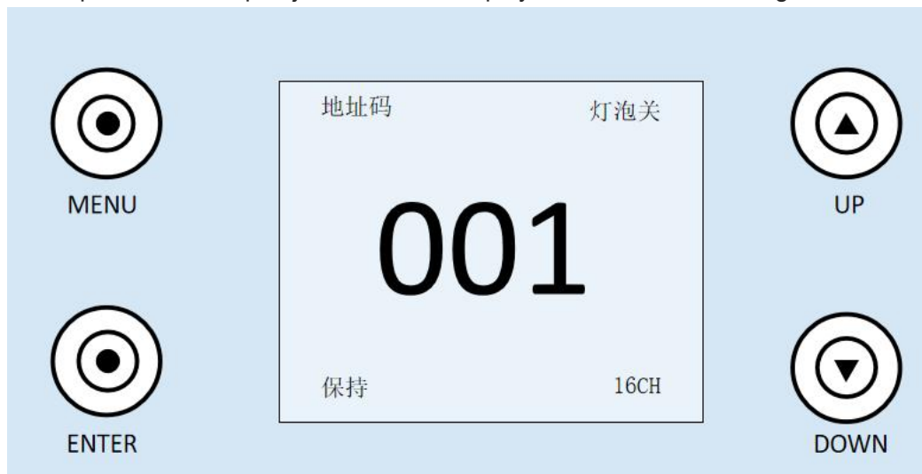
Figure 3 Schematic diagram of the four-button display panel
