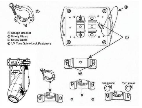
Regardless of the rigging option you choose for your fixture, always be sure to secure your fixture with a safety cable. The fixture provides a built-in rigging point for a safety cable on the hanging bracket as illustrated above. Be sure to only use the designated rigging point for the safety cable and never secure a safety cable to a carrying handle.
