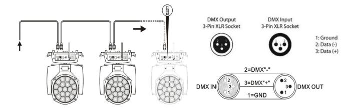
For installations where the DMX cable has to run a long distance or is in an electrically noisy environment, such as in a discotheque, it is recommended to use a DMX terminator. This helps in preventing corruption of the digital control signal by electrical noise. The DMX terminator is simply an XLR plug with a 120  $\Omega$  resistor connected between pins 2 and 3,which is then plugged into the output XLR socket of the last fixture in the chain. Please see illustrations below.
