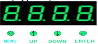
After boot, press MENU to switch menu, press UP (up) DOWN (down) to select the value size, and then press ENTER(OK) to save, no key operation after 30 seconds automatic screen saver, press any key to activate.
